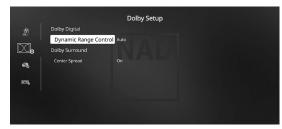
**Dynamic Range Control:** You can select the effective dynamic range (subjective range from soft to loud) for playback of Dolby Digital soundtracks. For fully cinematic effect, always select 100%, the default. Settings of 75%, 50%, and 25% progressively reduce dynamic range, making soft sounds comparatively louder while limiting the peak loudness of loud ones.
