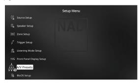
3 At "A/V Presets" page, set "Preset: 1" to the following conditions – use [▲/▼] to select "Yes" and press [ENTER] to confirm selection and move on to the next setting.
