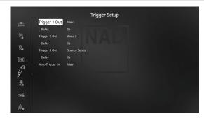
The M17 features three configurable +12V DC Trigger Output that can be used to activate a component or system it is fed into. A Trigger Input can also be configured to turn ON/OFF a section of M17.
