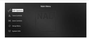
The Main Menu contains the menu options for "DSP Options", "Tone Controls", "Zone Controls", "System Info" and access to "Setup Menu".
