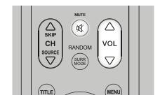
In addition to the Volume knob, use the HTRM 2's VOL [ $\blacktriangle/\blacktriangledown$ ] to adjust the "master volume" of the M17 raising or lowering the channels altogether. A momentary keypress will change the master volume by 0.5dB increments. If you hold down VOL [ $\blacktriangle/\blacktriangledown$ ], the master-volume change will "run-on" until the key is released.
