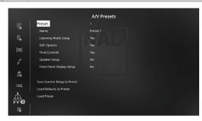
The M17's simple but powerfully flexible system of "AVV Presets" allows you to customize virtually every aspect of your audio-video playback, and recall them with a single key-press. The parameters "DSP Options" and "Tone Controls" accessible via the "Main Menu" together with "Listening Mode Setup", "Speaker Setup" and "Front Panel Display Setup" configurable through "Setup Menu" are stored together as a single A/V Preset.
