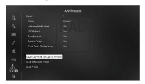
While at "Save Current Setup to Preset" menu line, use [▶] to save the above settings to Preset 1. Below OSD will be shown, affirming that the above settings are now saved to "Preset 1".
