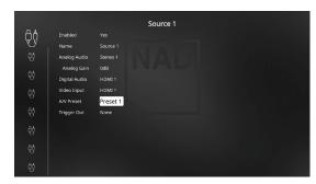
In the above example, "Preset 1" settings are allocated for Source 1. Whenever Source 1 is accessed, the "Preset 1" settings will be applied to Source 1. You can still manually override the assigned A/V Preset allocation in a specific Source with another Preset setting/number by way of pressing the appropriate remote control buttons.
