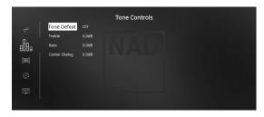
The M17 has three Tone Control levels – Treble, Bass and Center Dialog. Bass and Treble controls only affect the low bass and high treble leaving the critical midrange frequencies free of coloration. The Center Dialog ("Dialog" in the front panel display) control boosts the "presence" of the midrange region improving intelligibility of speech.
