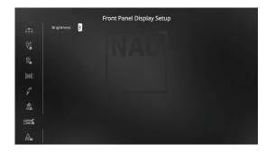
The brightness level of the front panel display can be adjusted. Level "3" is highest brightness level while "1" is the lowest.
