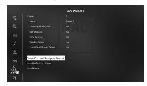
While at "Save Current Setup to Preset" menu line, use [1] to save the settings above to "Preset 2". When you recall "Preset 2" using the remote control (for HTRM 2, "A/V PSET"+ "2"), the above preset values allocated at "Preset 2" (preset settings as shown in the OSD captures at Step 4) will be recalled and effected at the current source.
