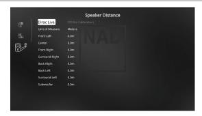
Your system's speaker distance settings are a subtle but important refinement of your setup. Informing the M17 of the loudspeaker-to- listener dimensions of each speaker automatically imposes the correct delays, optimizing imaging, intelligibility and surround-sound ambience. Enter your dimensions with precision within about 1 foot (0.3m).
