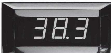
The digital display indicates the total-volume rotary angle as a percentage. The rotary angle is set by a separate potentiometer and is then displayed. The displayed values provide a volume reproduction of: 00.0...100.0%.
