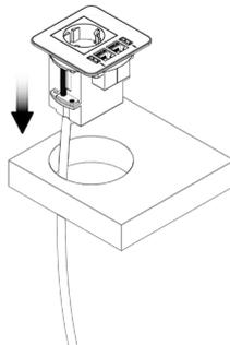
Once the hole has been cut to size, the product should simply slot into place. Make sure all cables are passed through the hole first.
