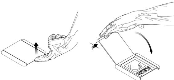
Open the product by simply pressing the button on the top of the flap. You can also open by just lifting up the flap. To close the unit, gently push the flap downwards until it clicks.
