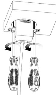
When the In-desk plate is situated in the hole, you can tighten the product in place by screwing the two Philips head screws at the bottom of the product.
