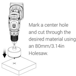
Mark a center hole and cut through the desired material using an 80mm/3.14in Holesaw.
