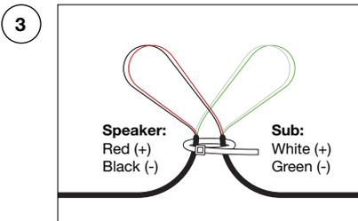
Use a Wire Stripper to remove the outside protective jacket to expose the four color-coded wires. Separate the wire loops as shown.
