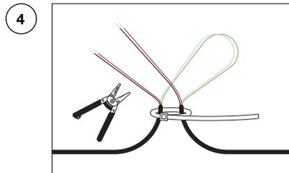
Cut the red (+) and black (-) wires with cable strippers and strip off 1 inch (25mm) of insulation from the wire ends to expose the copper conductor.
