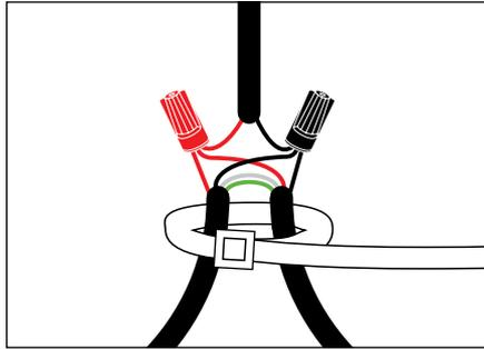
Combine and twist (clockwise) the red wires (see diagram) from the amp, speaker, and to the next speaker in the series. Secure these three wires using the provided silicone-filled wire connectors; Repeat procedure for Black wires.
