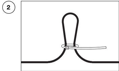
Use a wire tie (*not included*) to keep the wire loop intact and act as a strain relief.
