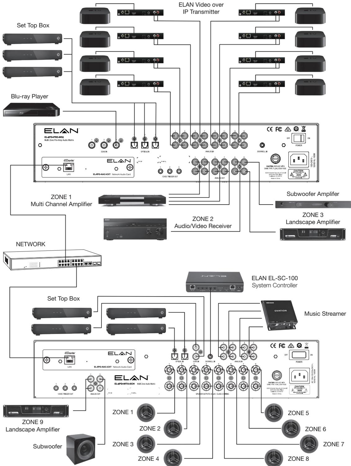
Adding the EL-IPD-NAC-EXT -Network Audio Card gives the ability to combine multiple chassis in to one system. Combine the EL-IPD-PRE-MSI Multi Zone Preamp Audio Matrix with the EL-IPD-AMP-EXT Multi Zone Audio Extender to add up to 8 zones of audio. Using Dante™ Audio Networking, the two chassis can be linked using standard networking equipment.
