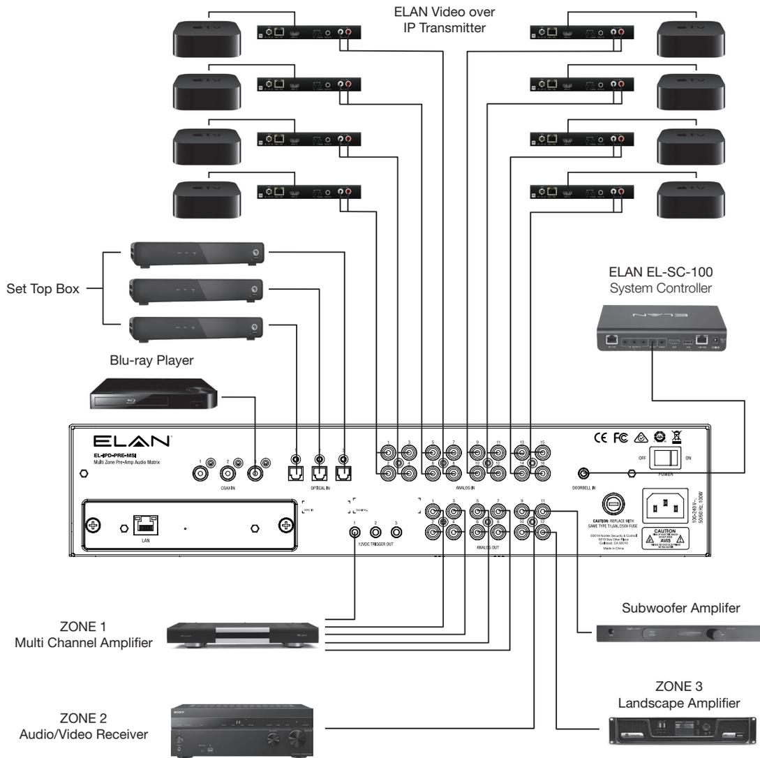
Adding the EL-IPD-NAC-EXT -Network Audio Card gives the ability to combine multiple chassis in to one system. Combine the EL-IPD-PRE-MSI Multi Zone Preamp Audio Matrix with the EL-IPD-MTX-8CH Multi Zone Audio Matrix to add up to 12 outputs and up to 12 inputs. Using Dante™ Audio Networking, the two chassis can be linked using standard networking equipment.
