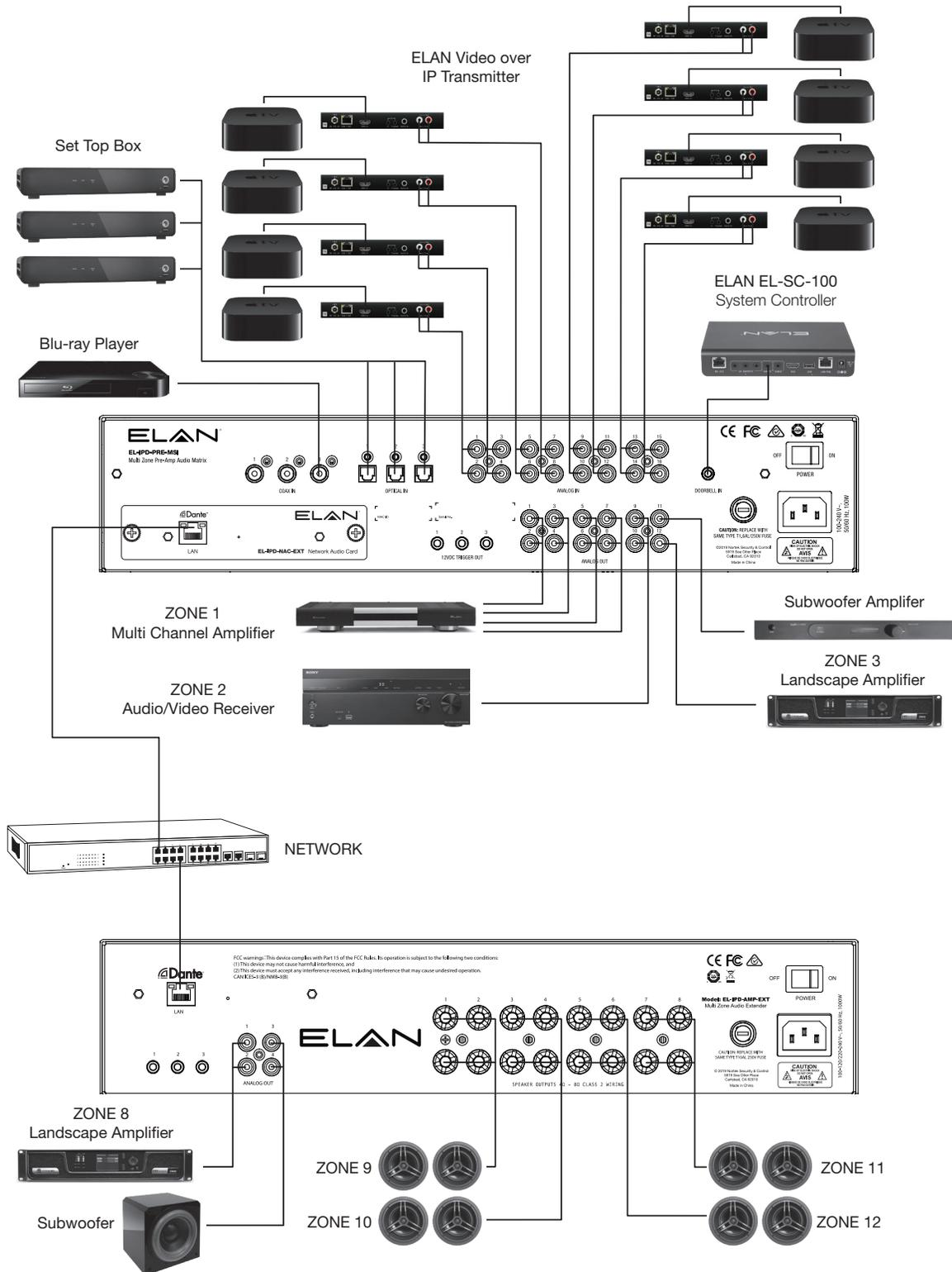
If remote sources are needed such as a TV's audio output, the EL-IPD-PRE-SSI Local Audio Source input device can be added to the system send audio over the network. Using Dante™ Audio Networking, the two devices can be linked using standard networking equipment. The EL-IPD-PRE-SSI is an additional source added to the direct input sources on the the main chassis.
